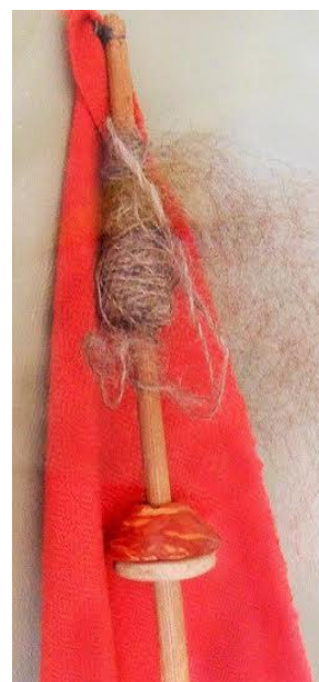
Figure 6.2 Spindle using two whorls to add weight for spinning of heavier yarns.
